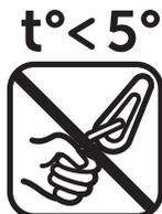
Install only at temperature above  $+5^{\circ}\text{C}$ !
